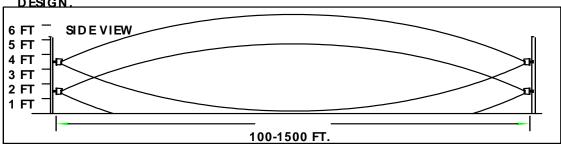
\* THE MICROWAVE SENSORS CAN BE MOUNTED IN A DUAL CONFIGURATION TO PROVIDE A GREATER PROBABILITY OF DETECTION.
