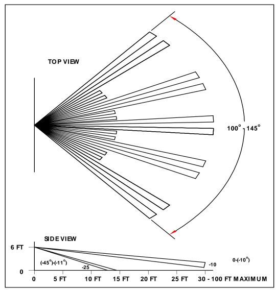
THE NUMBER, RANGE, AND PROJECTION ANGLES OF THE DETECTION BEAMS VARY DEPENDING UPON DESIGN.
