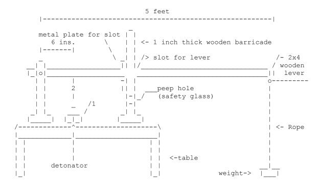
Notes: 1. Block- wood (10" x 10" x 6" or steel (6" x 6" x 6") with 3/8" diameter hole 1" deep.
