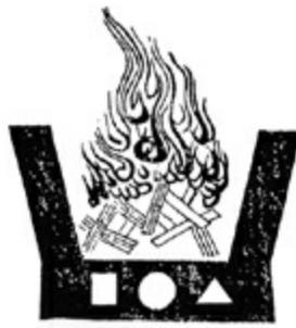
As shown in the drawing, embank the fire on three directions, with the walls facing your camp and the fire shining outward, toward the enemy. The height of the walls should be about 7 *shaku*. Put intakes into it to create airflow. The size can be changed according to your purpose. The appropriate position or distance that a fire should be in relationship to the camp is written in *Sonae no Sho*, the second scroll.
