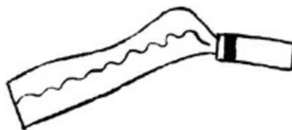
The clamping spike should be 1 *sun* in width and 2 *bu* in thickness. The handle should measure 8 *sun* long. The blade should be 3 *sun* wide and 5 *sun*, 5 *bu* long. This can reach to 6 or even 7 *sun*. Make a sharkskin sheath the length of 9 *sun*, 5 *bu*. Put a hole at the tip of the sheath and then connect a thieves' gimbal lantern onto it. Wear the tool on the left.
