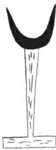
The type of drill described in the *Bansenshūkai* and used to cut out small holes.
