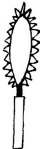
Make it 2 *sun* in width. The handle should be 1 *shaku*, 2 *sun*. The blade should be 1 *shaku*, 2 *sun*. This tool is used to cut bamboo and wood.
