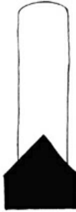
Change the length according to the depth of water. The upper white section is a thin plate of brass 1 *sun* wide and 1 *bu* thick. The bottom section is made of gold and is 1 *sun* long, 1 *sun* wide.
