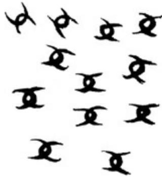
Each caltrop is 1 *sun*, 5 *bu* long. The above shape is in case you use iron. If you use bamboo, cut it into pieces of 2 *sun* long, and connect them so that one point always stands upright with the shards left, as sharp as when they are cut.
